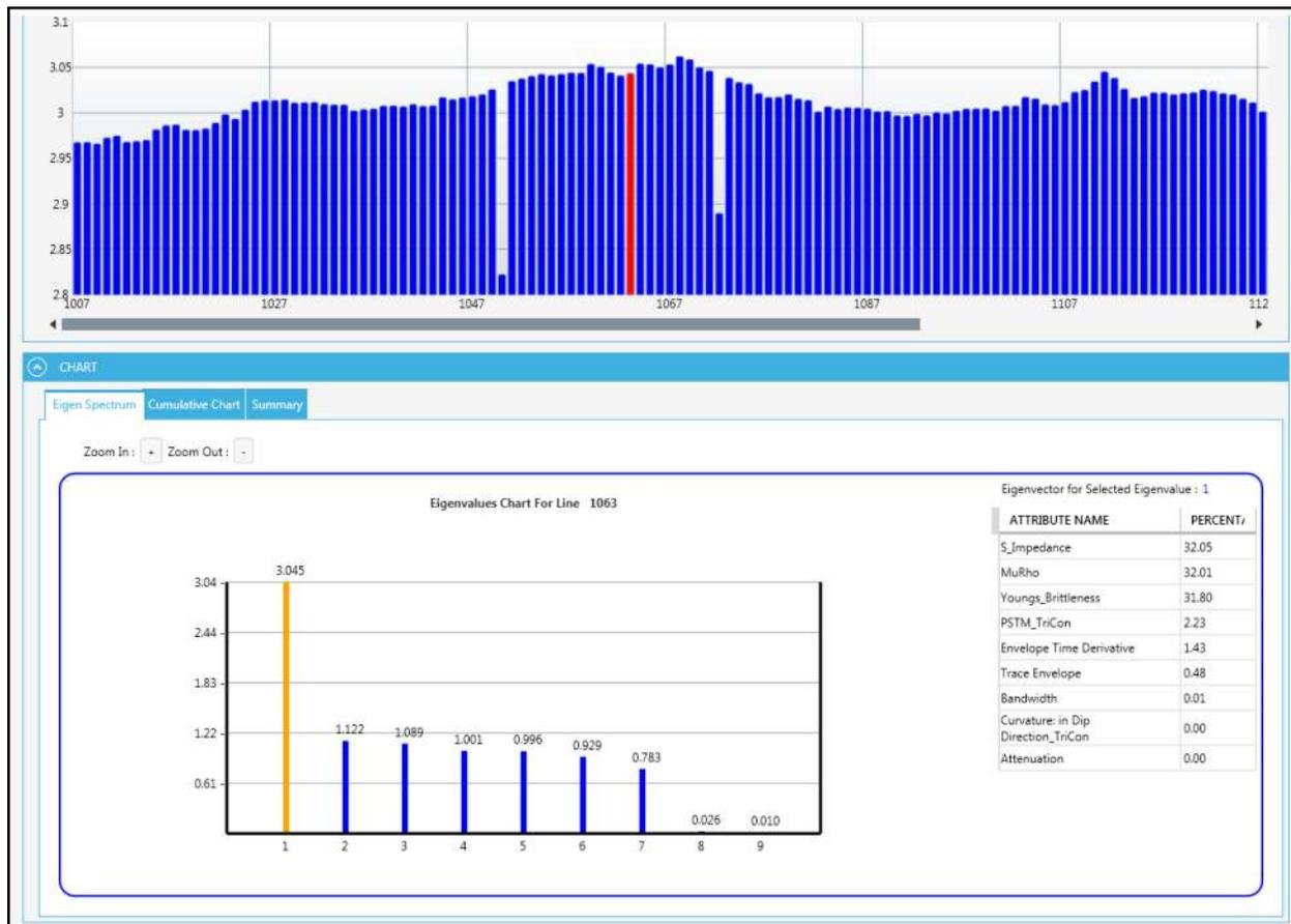
Figure 1—Principal Component Analysis (PCA) results displayed in Paradise® with top histograms displaying highest eigenvalues for 3D inlines and bottom portion displaying the highest eigenvalue at the red histogram location above. The bottom right display indicates the percentage contribution of the attributes in the first principal component.
