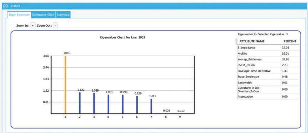
**FIGURE 1.** PCA in the Paradise software displays highest eigenvalues for 3-D inlines in the upper portion with selected largest eigenvector (red); then all eigenvalues for the inline are shown in the lower left from largest (yellow) to smallest. The lower right portion shows the attributes and their proportion for the eigenvector corresponding to the largest eigenvalue. (Source: Geophysical Insights)
