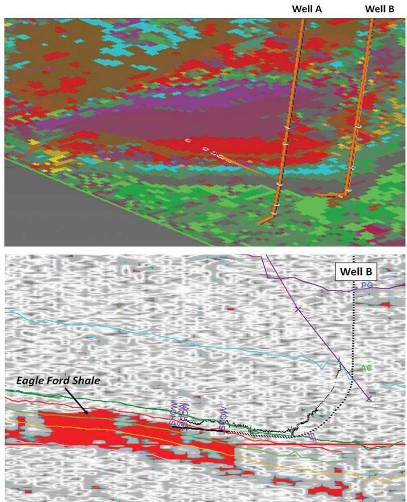
**FIGURE 2. (Top) SOM classification from the Paradise software shows the Eagle Ford interval displaying dry hole Well A and good Well B; (bottom) vertical seismic display through Well B indicates shows as the well entered the Eagle Ford interval. (Source: Geophysical Insights)**
