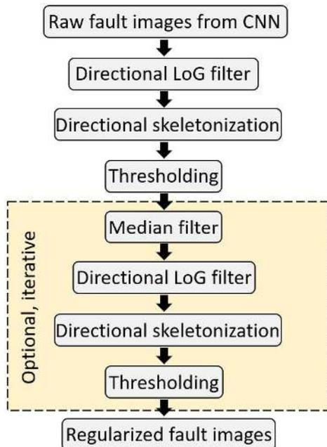
Figure 2. The regularization workflow used to improve the fault images after CNN fault detection.
