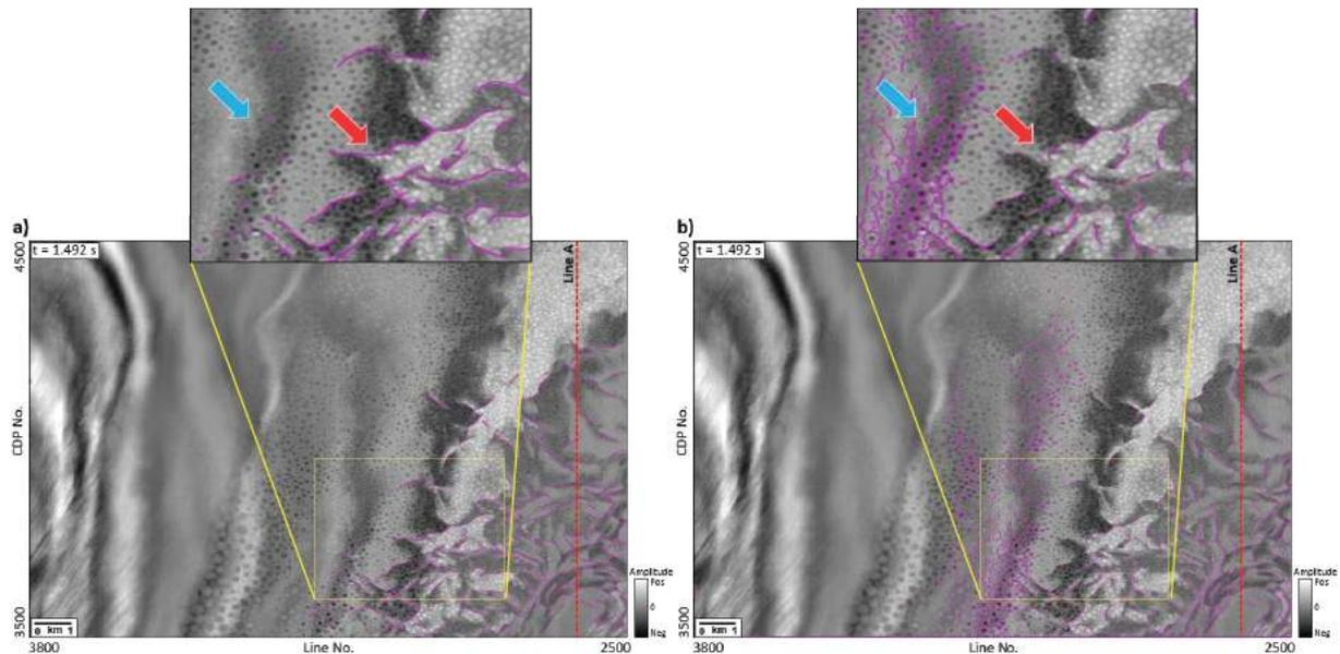
Figure 7. Seismic amplitude along  $t = 1.492s$  co-rendered with a) faults generated from the proposed workflow and b) faults generated from using coherence in lieu of raw CNN output in the regularization workflow. Blue arrows indicate regions with coherence anomalies not caused by faults. Red arrows indicate faults images are more continuous from the proposed workflow.
