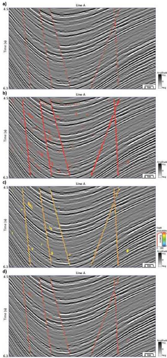
Figure 3 (Left.) Line A from the synthetic data showing seismic amplitude with a) artificially created faults highlighted in red; b) raw output from CNN fault detector; c) CNN detected faults after directional LoG and skeletonization; and d) final fault after thresholding.
