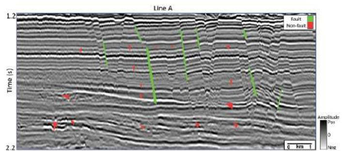
Figure 6. A vertical slice from the field seismic amplitude data with manually picked regions for training the CNN fault detector. Green regions represent fault and red regions represent non-fault.
