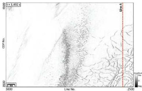
Figure 5. Coherence attribute along  $t = 1.492s$ . Coherence shows discontinuities not limited to faults, posing challenges to obtain only fault images.
